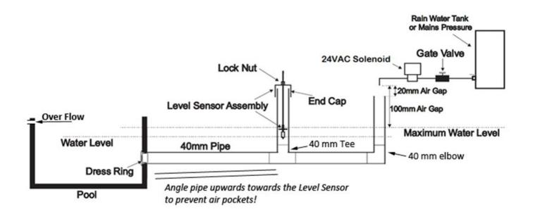
Fill Pool or Spa to correct operating level before setting water level sensor.
