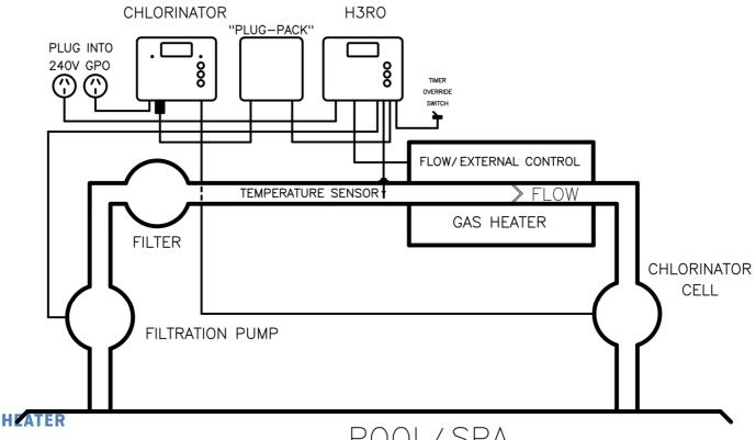
Connect the heater cable from the controller output marked HEATER to the heaters flow or pressure switch, check with heater manufacturer for correct interlocking procedure, see picture for typical connection set-up. Note damage caused by incorrect connections will void warranties.
