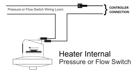
Internal connection to pool heater (check with heater manufacturer).
